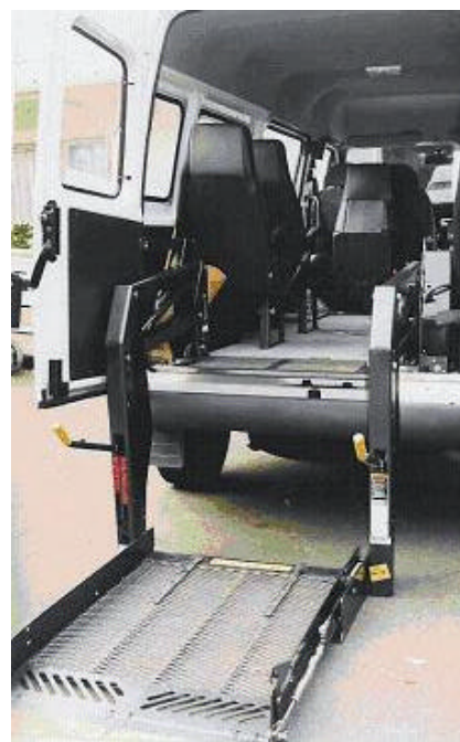
Above: Hoist in down position – no guard to prevent inadvertent egress.
