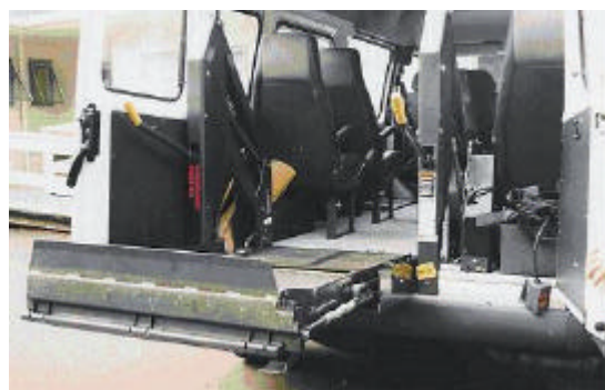
Above: Hoist in horizontal position ready to receive a wheelchair
