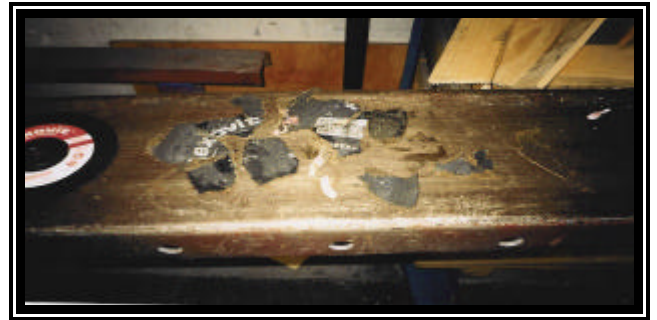
Pieces of the disintegrated disc (rated at 4,200 rpm and designed for a cut-off saw), after it was used on a 230 mm portable angle grinder rated at 6,600 rpm.
