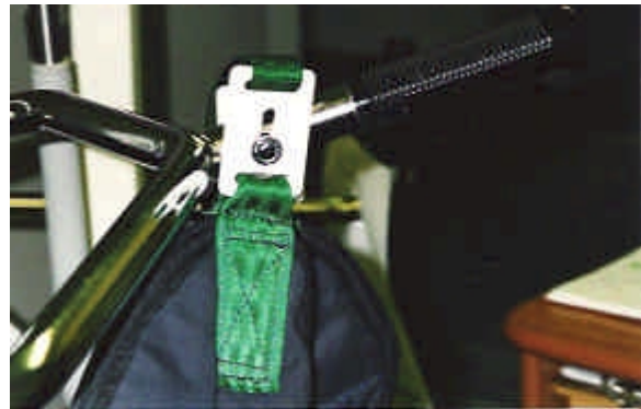
Incorrect attachment of the buckle on the stud head.
