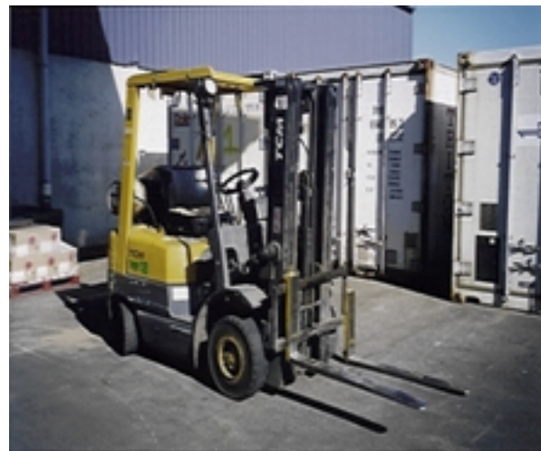
View of forklift with the load guard/backrest removed.
