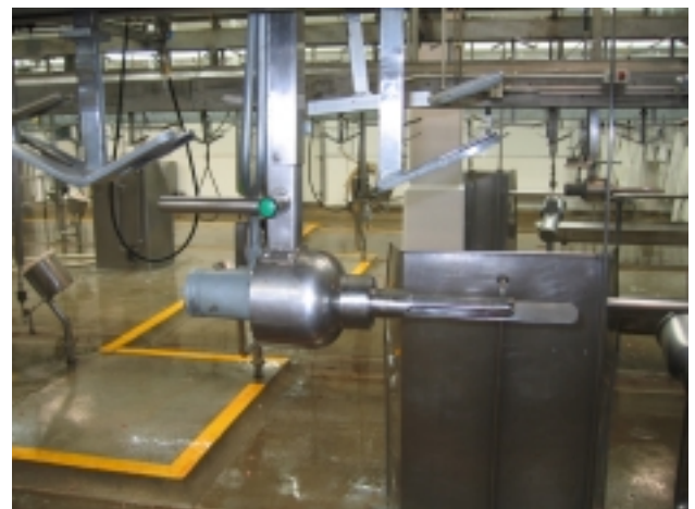
A brisket roller of the type involved in this accident.
