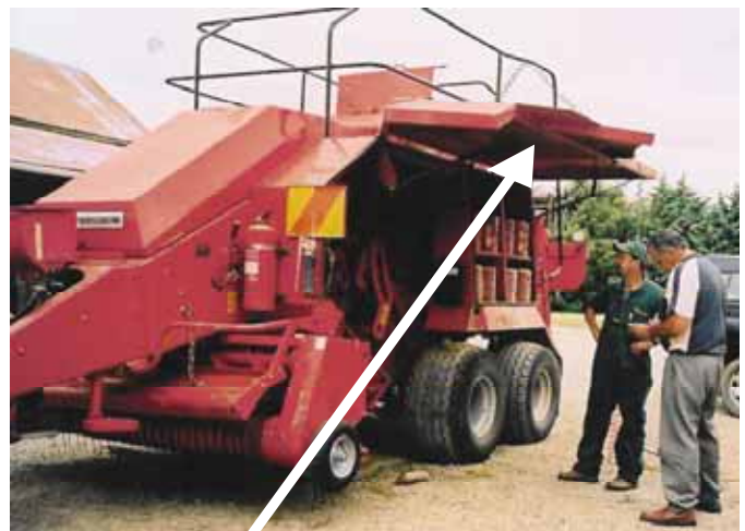
Guard that had been lifted to oil the chains
